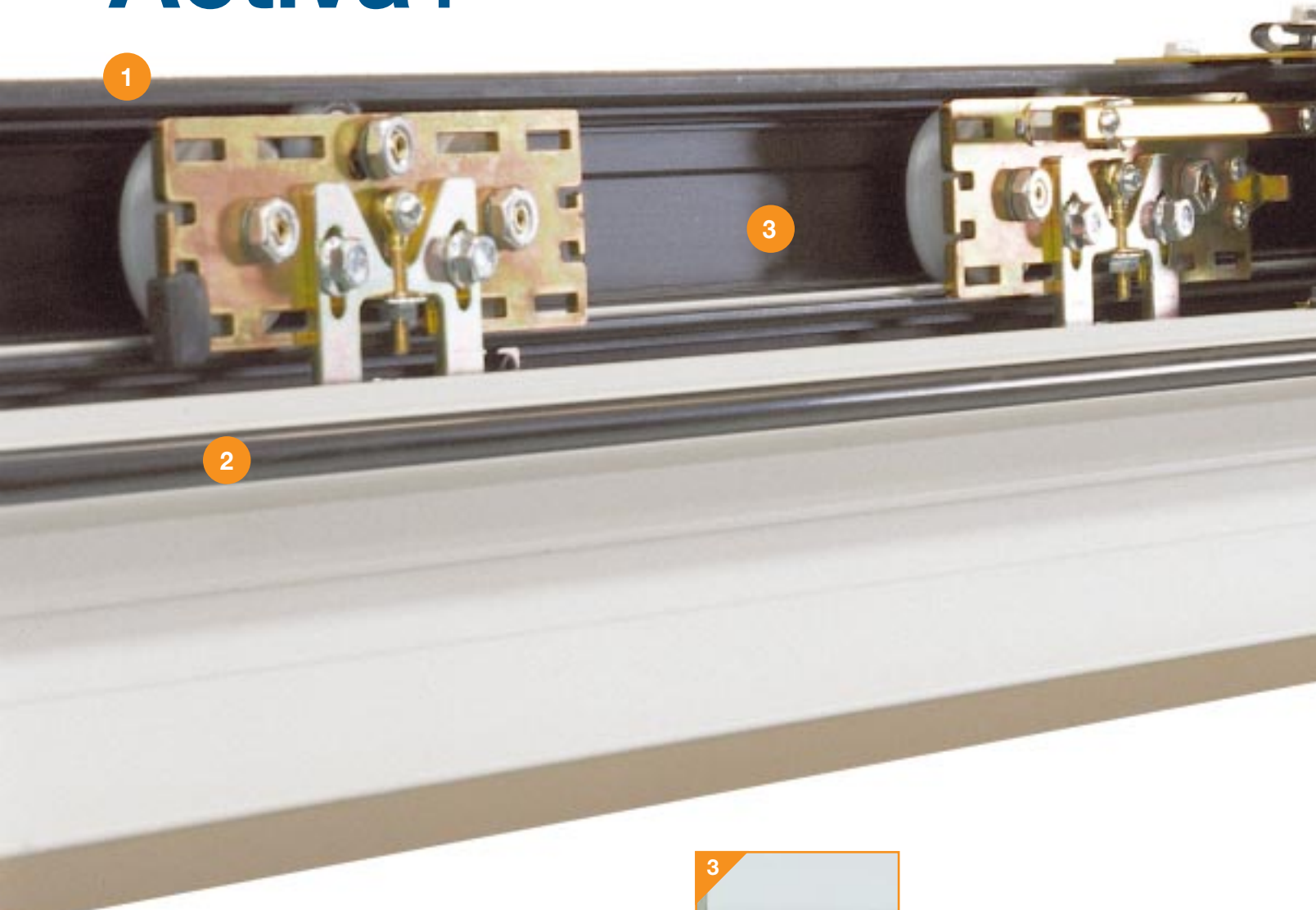
Independent track rail Insulated and easy to replace, provides smooth and silent operation
