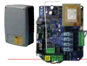
ABT2001W T2 Wi-Fi control board (for 1 or 2 R50) with thrust regulator and MASTER Wi-Fi. With box. See pages 116, 142 and 143
